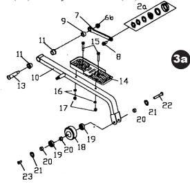
3. Slide the Bolts (12, 13) through the hole of the Foot Pedal Mount Tubes (10) and screw into the Crank (7). Must screw on counter clockwise. Secure both Bolts (12, 13) with Nuts (6a, 6b). Do not forget to place the Plastic Spacer (9) in first. (See 3a above).
